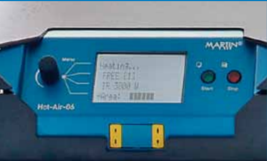
Operator friendly display. Simple menu structure, using just one knob.
